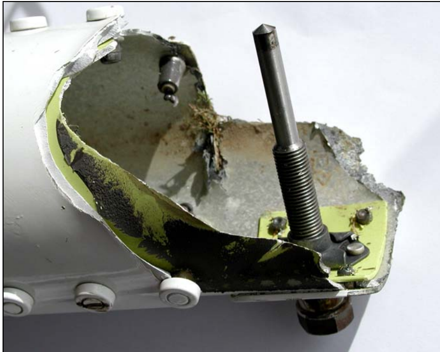
Photograph of skid fracture caused by a combination of exfoliation, galvanic and stress corrosion ( Photo by Tony Horan )
